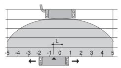
5 mm misalignment tolerance after setting
