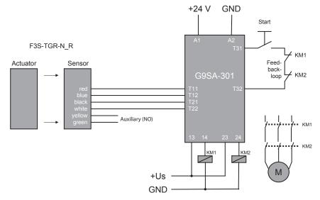
Series connection Application, up to 6 Sensors with G9SA-301
