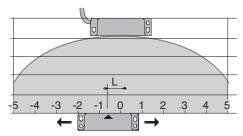
5 mm misalignment tolerance after setting
