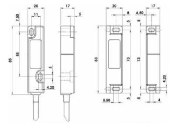
Wide Sensor (Sensor/Actuator) F3S-TGR-NWPR
