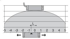
5 mm misalignment tolerance after setting
