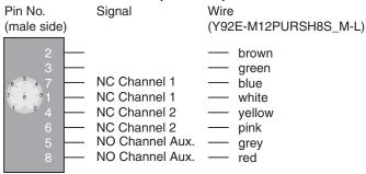
Note: If the auxiliary circuit is not fitted or not used then cut and discard the yellow/green or grey/red conductors.
