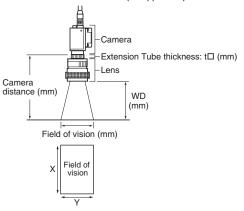
Note: 1. The lengths of the fields of vision given in the optical charts are the lengths of the Y axis.2. The vertical axis represents WD for small cameras.
