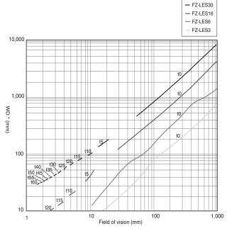
$^{\star}\,$  The vertical axis represents WD, not installation distance.
