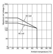
Ambient Temperature vs. Must Operate and Must Release Voltage G2R-1
