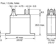
Mounting Holes (BOTTOM VIEW) Tolerance: ±0.1 mm
