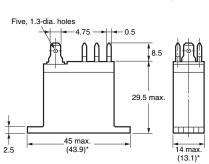
Mounting Holes (BOTTOM VIEW) Tolerance: ±0.1 mm
