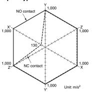
Sample: G2RL-14 12 VDC Number of Relays: 5 pcs Test conditions: Shock is applied in ±X, ±Y, and ±Z directions three
