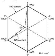
Sample: G2RL-14 12 VDC Number of relays: 5 pcs Test conditions: Shock is applied in  $\pm X$ ,  $\pm Y$ , and  $\pm Z$  directions three times each with without energizing the relays to check the number of
