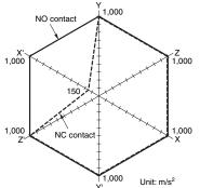
Sample: G2RL-24 12 VDC Number of relays: 5 pcs Test conditions: Shock is applied in  $\pm X$ ,  $\pm Y$ , and  $\pm Z$  directions three times each with without energizing the Relays to check the number of malfunctions.
