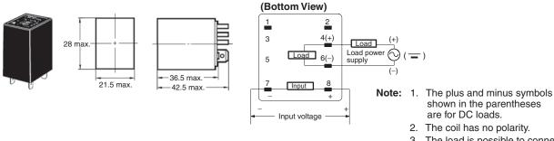
The load is possible to connect either + side or - side.
