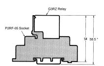
\* Indicates a value when using the PFP-□N Supporting Rail. The value is 67.5 when using the PFP-□N2.
