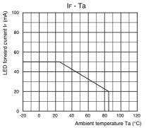
Continuous load current vs. Ambient temperature
