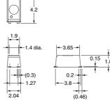
Unless otherwise specified, the dimensional tolerance is  $\pm$  0.1 mm.
