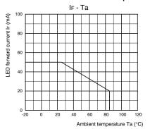
Continuous load current vs. Ambient temperature
