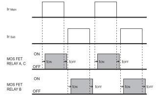
\* Both MOS FET relay A, C and MOS FET relay B may be ON at the same time. For that reason, even if pins 4, 5 and 6 are all connected, please design the circuit so that equipment damage does not occur.
