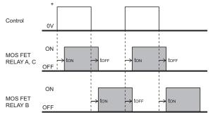
\* Both MOS FET relay A, C and MOS FET relay B may be ON at the same time. This products is recommended to use with dry switching (No Load & No Source when switching) to prevent short circuiting.
