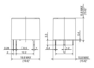
PCB Mounting Holes (Bottom View) Tolerance: ±0.1 mm Unless specified
