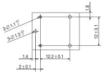
Terminal Arrangement/Internal Connections (Bottom View)
