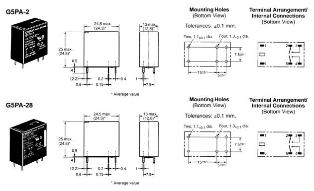
ALL DIMENSIONS SHOWN ARE IN MILLIMETERS. To convert millimeters into inches, multiply by 0.03937. To convert grams into ounces, multiply by 0.03527.
