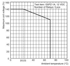
Note. The maximum coil voltage refers to the maximum value in a varying range of operating power voltage, not a continuous voltage.
