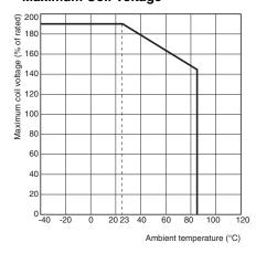
Note. The Maximum coil voltage refers to the maximum value in a varying of operating power voltage, not a continuous voltage.
