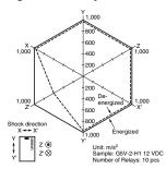
Conditions: Shock is applied in ±X, ±Y, and ±Z directions three times each with and without energizing the Relays to check the number of contact malfunctions.
