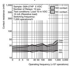
Operating frequency (×10<sup>4</sup> operations) The tests were conducted at an ambient temperature of 23°C.
