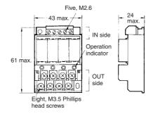
Note: Do not reverse the coil polarity.
