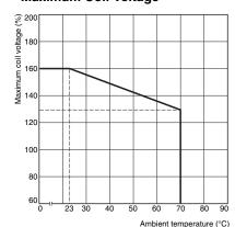
Note. The maximum coil voltage is the maximum voltage that can be applied to the relay coil.
