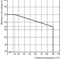
Note. The maximum coil voltage refers to the maximum voltage in a varying range of operating power voltage, not a continuous voltage.
