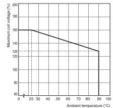
Note. The maximum coil voltage refers to the maximum voltage in a varying range of operating power voltage, not a continuous voltage.
