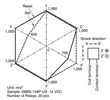
Test Conditions: Shock is applied in  $\pm X$ ,  $\pm Y$ , and  $\pm Z$  directions three times each with and without energizing the Relays to check the number of contact malfunction.
