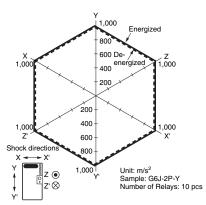
Test Conditions: Shock is applied in ±X, ±Y, and ±Z directions three times each with and without energizing the Relays to check the number of contact malfunctions.
