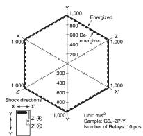
Test Conditions: Shock is applied in  $\pm X$ ,  $\pm Y$ , and  $\pm Z$ directions three times each with and without energizing the Relays to check
