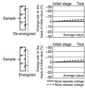
The test was conducted at an ambient temperature of 23°C. \*1. \*2. The contact resistance data are periodically measured reference values and are not values from each monitoring operation. Contact resistance values will vary according to the switching frequency and operating environment, so be sure to check operation under the actual operating conditions before use.
