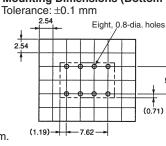
Mounting Dimensions (Bottom View) Terminal Arrangement/ Internal Connections
