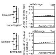
Note 1: The test was conducted at an ambient temperature of 23°C. The contact resistance data are periodically measured reference values and are not values from each monitoring operation. 2: Contact resistance values will vary according to the switching frequency and operating environment, so be sure to check operation under the actual operating conditions before use.
