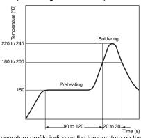
(The temperature profile indicates the temperature on the circuit board.)
