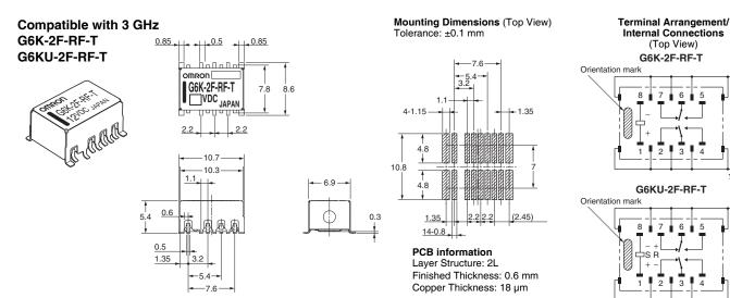
Note 1. Each value has a tolerance of ±0.3 mm.
