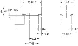
Note: Each value has a tolerance of ±0.3 mm.
