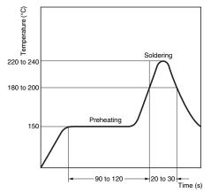
Note: The temperature profile indicates the temperature on the circuit board.
