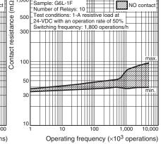
Note: 1. The tests were conducted at an ambient temperature of 23°C. The contact resistance data are periodically measured reference values and are not values from each monitoring operation. Contact resistance values will vary according to the switching frequency and operating environment, so be sure to check operation under the actual operating conditions before use. 2.
