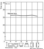
(Note.)The mounting direction A' deteriorates switching performance.
