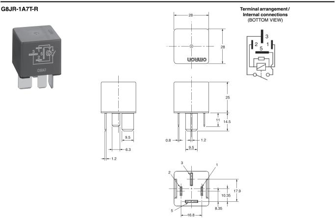
\* Tolerance unless otherwise specified Less than 1 mm: ±0.1 mm Less than 1 to 3 mm: ±0.2 mm
