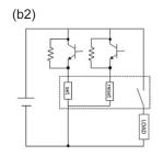
OMRON recommends coil driver circuit (b) and (c) for coil surge suppression. However the circuit (d) is not recommended because it may negatively affect the durability performance.
