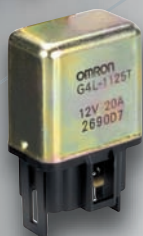
G4L(1a) JASO Rated 20 A Inrush 100 A
