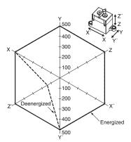
The value at which malfunction occurred was measured after applying shock to the test piece 3 times each in 6 directions along 3 axes.
