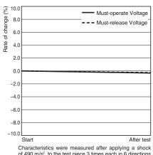
Characteristics were measured after applying a shock of 490 m/s<sup>2</sup> to the test piece 3 times each in 6 directions along 3 axes. The percentage rate of change is the average value for
