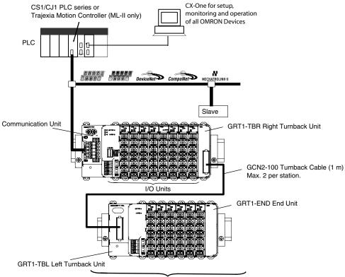
Up to 64 I/O Units can be connected to a Communication Unit.
