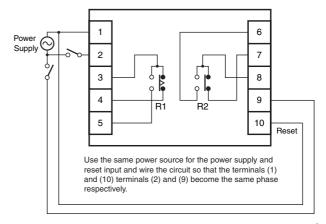
Note: The R2 relay can be switched between instantaneous and time-limit contacts and thus the contact symbol is shown as follows: 🖟
