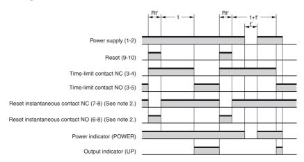
**Note: 1.** t is the set time, Rt' is the reset application time, and t' is the power interruption time.
