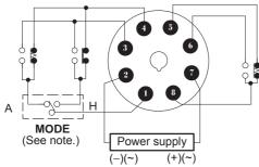
Note: The output contact can be set to either instantaneous or time-limit contact using the output type selector located at the upper right corner of the front panel.
