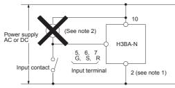
**Note: 1.** Power supply terminal 2 is a common terminal for the input signals (G, S, R) to the Timer. Never use terminal 10 as the common terminal for this purpose, otherwise the internal circuit of the Timer may be damaged.
