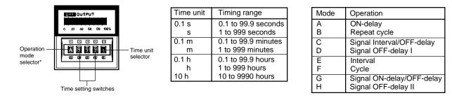
Note: \*Operation mode selector not included with ON-delay only models.
