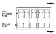
Fig. 2 Wire Connection Holes and Release Holes
