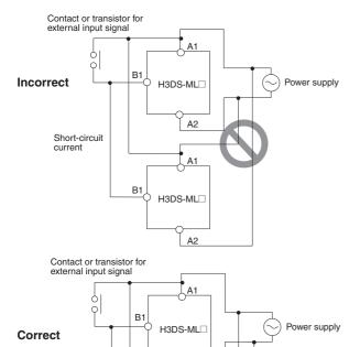
The H3DS Series is provided with a transformerless power supply system.
