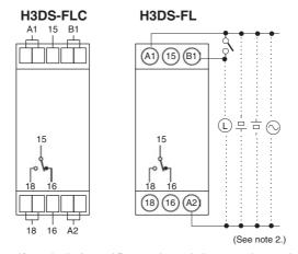
Note: 1. If voltage is applied to terminal B1, or if terminals A1 and B1 are shorted, the operating mode is switched to flicker-ON start mode. If these terminals are disconnected, the mode switches to flicker-OFF start mode.
