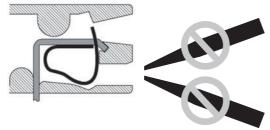
Do not move the screwdriver side to side in the clamp hole. The clamp spring may be deformed if the screwdriver is moved sideways.
