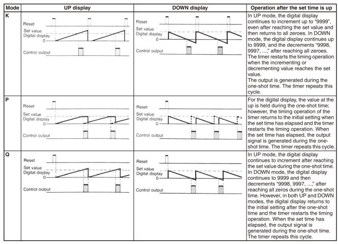
Note: 1. When a rated time of 99 min 59 s or 99 h 59 min is selected, the overflow values of the digital display when using the DOWN (countdown) function will be indicated as 9959, 9958, 9957, ... in modes F, K, and Q.
