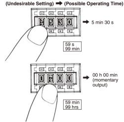
5. When operating the built-in selector switches of the H5AN-4DM Timer with a backup power supply function for memory protection, it is necessary to reset (either externally or manually) the timer at the time the power is applied. Also when this type of timer is connected to a device (or manually) this must also be done when power is applied for the first time.
