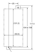
M4 tapping screws provided. Approximate pilot hole dimensions: Panel thickness of 0.8 to 1.2 mm: 3.6 mm dia. Panel thickness of 1.6 to 4.0 mm: 3.7 mm dia.
