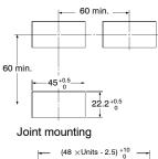
Waterproofing is not possible for joint mounting.
