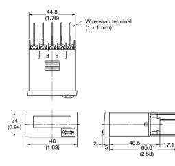
The wire-wrap terminals have a cross sectional dimension of 1x1 mm. Select one of three guages of wire from the table at right. Also listed in the table is the appropriate wiring hardware
