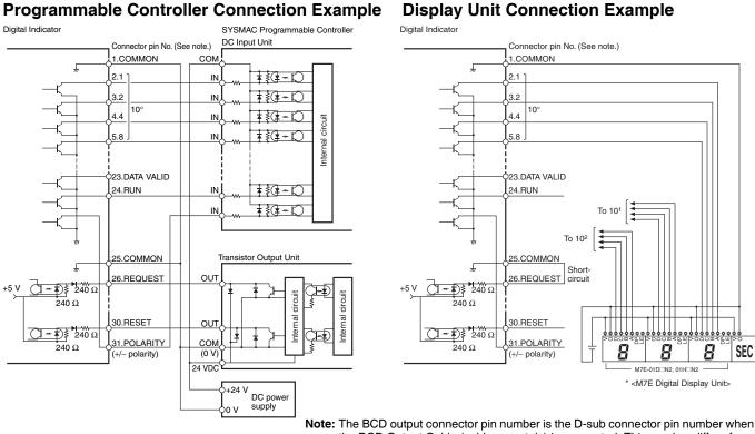
Intel BCD output connector pin number is the D-sub connector pin number when the BCD Output Cable (sold separately) is connected. This number differs from the pin number for the Digital Indicator narrow pitch connector (manufactured by Honda Tsushin Kogyo Co., Ltd.).
