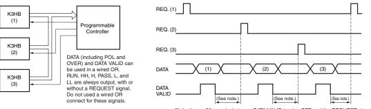
Note: Leave 20 ms min. between DATA VALID turning OFF and the REQUEST signal.
