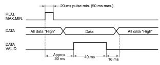
The data is set in approximately 30 ms from the rising edge of the REQUEST signal and the DATA VALID signal is output. When reading the data from a Programmable Controller, start reading the data when the DATA VALID signal turns ON. The DATA VALID signal will turn OFF 40 ms later, and the data will turn OFF 16 ms after that.
